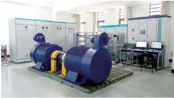
Experimental Platform of Low-speed Permanent Magnet Fan-driven Generator System
